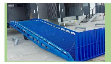
Mobile ramps RL-MR that is special equipment which allows forklift to load/unload trucks and railway wagons from ground level (zero). So, it acts as movable bridge, which could be adjustable in its height, thanks to hydraulic system and act as connection between ground and truck levels.
