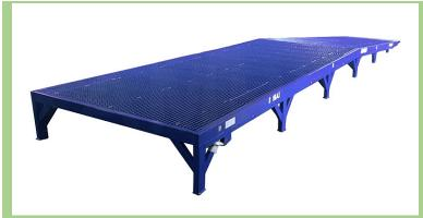
This is a special designed truck ramp for loading / unloading commercial vehicles at standard dock gates of modern warehouses. Our equipment helps to eliminate deference in heights of commercial vehicles (550-650 mm) and height of dock gates, dedicated for big semi-trailers (1100-1300 mm).
