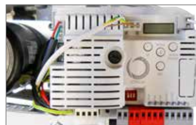
CT102 24 control board with integrated receiver
