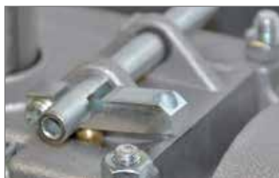
External release for an easy manual unlock from outside
